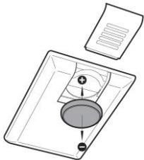
Slide the remote-control battery compartment cover downwards and remove the battery from the remote control. Insert the new battery (plus facing downwards) and slide the cover back on.
